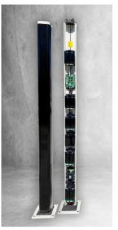
AVANTGARDE-DT is a high security active dual technology (DT) barrier enclosed in two tamper protected extruded aluminum columns equipped with Sicurit last generation of digital patented bi-directional infrared and brand new K-Band microwave technology, all within one unit.
